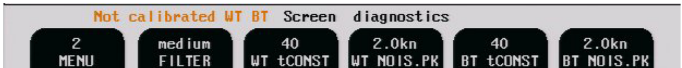
Screen diagnostics, Menu 2, filtering/averaging.
